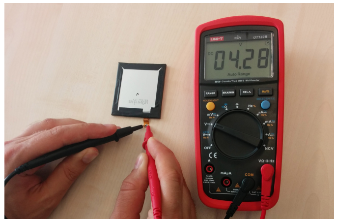
Fig. 9. Measuring the idle voltage of a fully loaded Nexus 5 battery.
