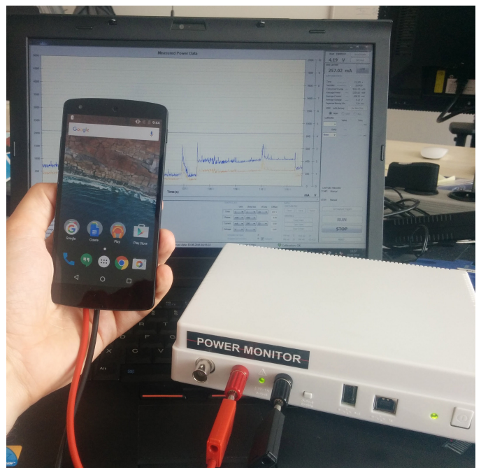
Fig. 10. Nexus 5 connected to the Monsoon Power Monitor.
